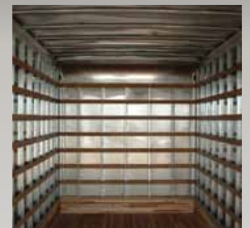
Dry Freight shown with optional translucent roof and optional wood slat lining
