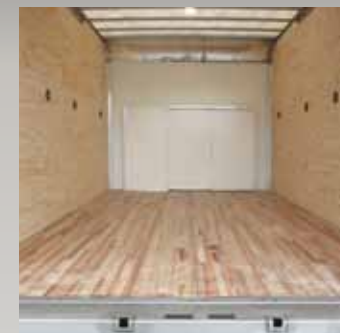
Citi-Van shown with standard plywood liner, tie rings, optional translucent roof and laminated hardwood floor
